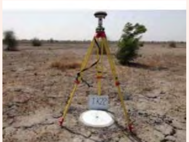
Masinga Dam - Bathymetric survey/ground controls
