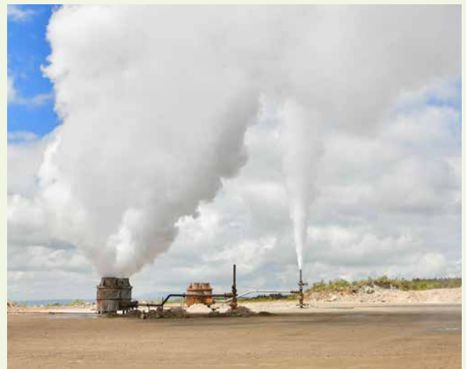
Recently drilled geothermal discharging well
